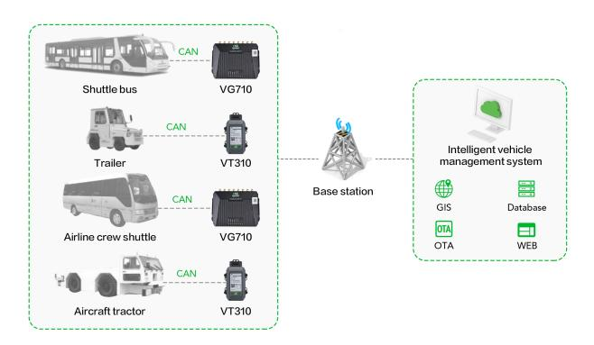
InHand Networks' VG710 smart vehicle gateway connects to the vehicle's ECU and reads related data into the gateway. Real-time vehicle location can be grasped through
