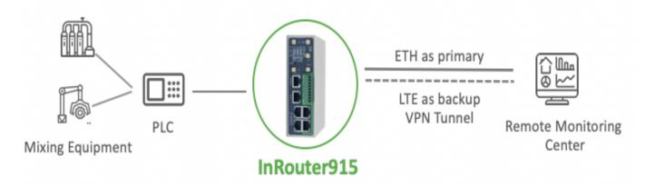
The monitoring system of concrete mixing equipment consists PLC, edge computing gateway InRouter915 and cloud monitoring center.
