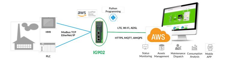
The platform can manage operation status data of heat supply stations, such as inflow water temperature, outflow water temperature, inflow water pressure, outflow water pressure, operation status of the compressor, leakage, temperature threshold value, activated status, alarm, etc.
