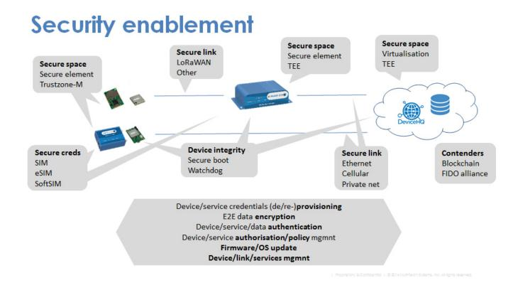
National wide networks targeting internet of things such as critical infrastructure, confidential personal data or critical functions for the society has a special need for secure communication. This has been solved by several layer of encryption:
