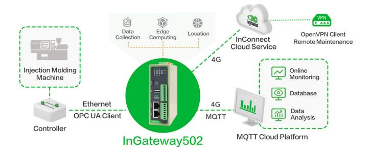
Onsite injection molding machines are connected to the IG502 via Ethernet ports. The IG502
